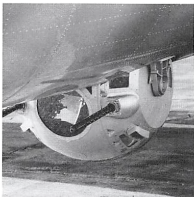
The ball (belly) turret of a B-17. Howard once said that during combat it seemed like there was just a small piece of glass between him and the ground.
